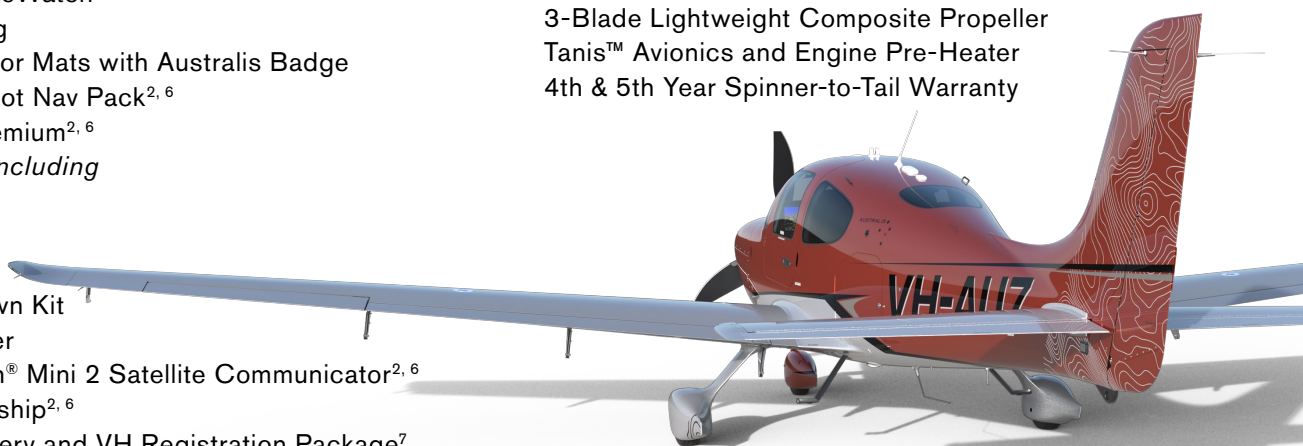
SR22 Australis shown with optional 3-Blade Lightweight Composite Propeller and Certified Flight Into Known Ice System
