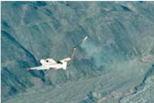
**Rocket and Parachute Extraction** - When the CAPS activation handle is pulled, the cable causes the rocket to ignite and dislodges the Rocket Assembly CAPS cover located behind the baggage compartment. The rocket extracts the deployment bag containing the packed parachute from the airplane. The deployment bag protects the parachute until it is away from the airplane and ensures the parachute will deploy in an orderly fashion.
