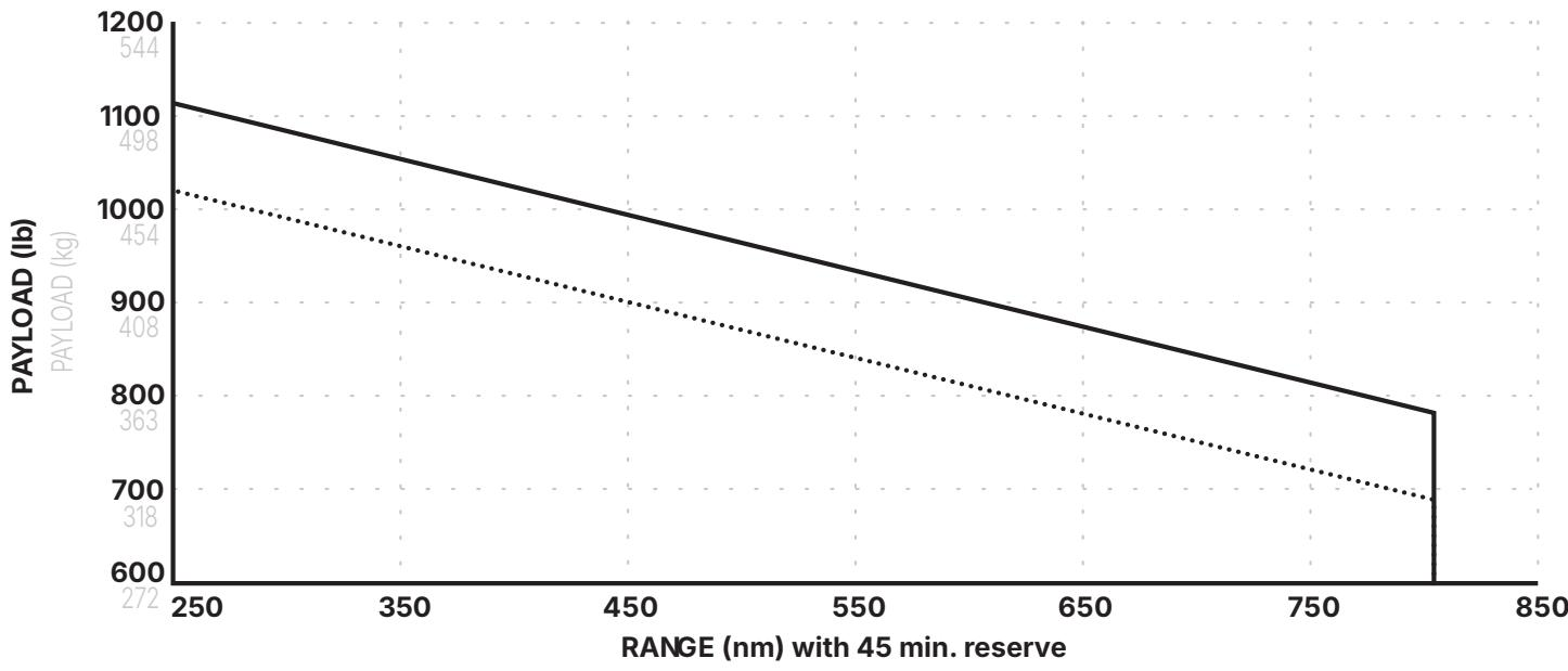
+1 lb (.45kg) Payload or Equipment = -1.7 NM
